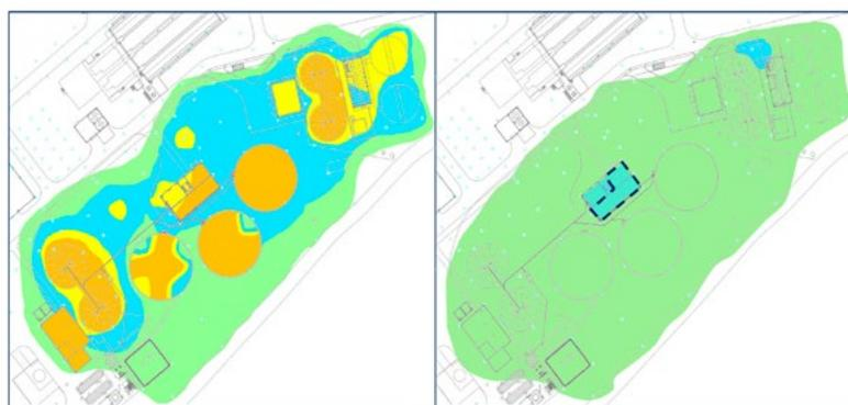
Figure 5. Concentrations of H<sub>2</sub>S (left) y relative humidity (right) in sludge line.
